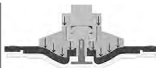
Figure 2: Compressor for Advantage 2.0 actuator
