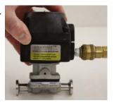
6. Install new diaphragm. Engage the threads of the diaphragm into the tube nut by rotating clockwise. Rotate the diaphragm until hard stop or heavy resistance is achieved and additional force does not significantly rotate the diaphragm into the compressor. See "PTFE Diaphragm Installation" instruction sheet for additional detail.
