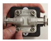
10. Tighten the bonnet fasteners in a crisscross pattern. Make multiple criss-cross passes to build up torque to the final table value. Make additional crisscross passes using final table values to evenly tighten each fastener to within 5% of torque value.
