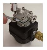
7. Back off (no more than 1/2 turn) until the bolt holes in diaphragm and the bonnet flange
