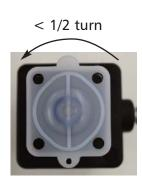
4. Unscrew the diaphragm from the compressor by turning counterclockwise..
