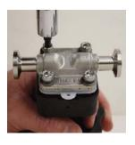
6. Back off (no more than 1/2 turn) until the bolt holes in diaphragm and the bonnet flange align.
