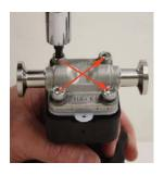
each fastener to within 5% of torque value.
